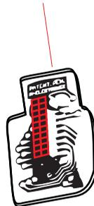
Close the Control box and stick a new label over the 5th screw
