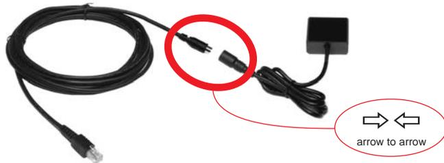
To achieve maximum water resistance put a heat shrink tube (included) on the connector. Use a strong heater for the tube to shrink and conform to connector size. The tube can be torn apart when the sensor requires disconnection.
